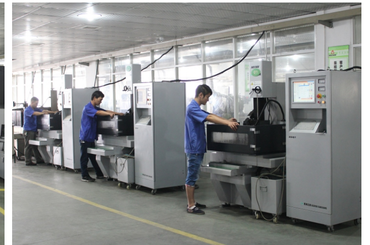
Medium speed wire cutting machines(11 sets)
