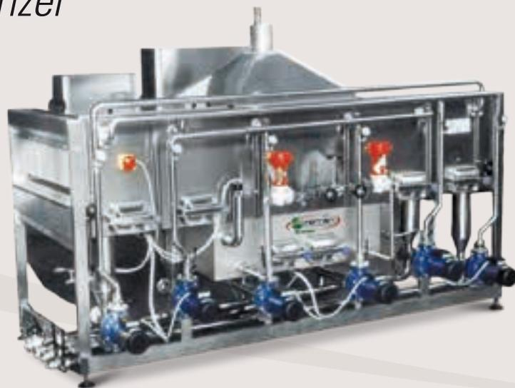
*The pasteurization tunnel are constructed entirely of stainless steel and are equipped with a number of pumps that allow a perfect balance of temperature and a complete heat recovery minimizing energy consumption.*
