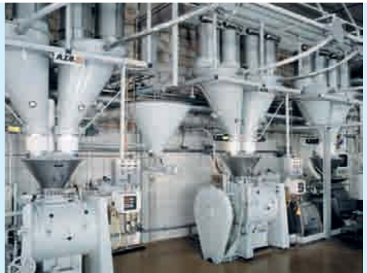
Recipient hopper for flour and sugar in a system with central weighing system
