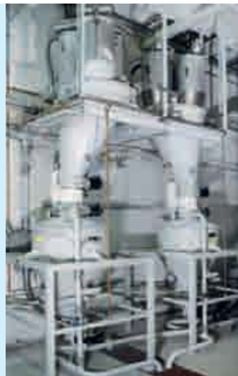
Central weighing station for long-lasting bakery products
