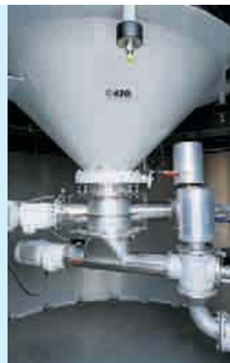
Dust free product intake and clean frame skirt through suction conveying: left – vibration bottom with dosing screw, right – with dosing rotary valve
