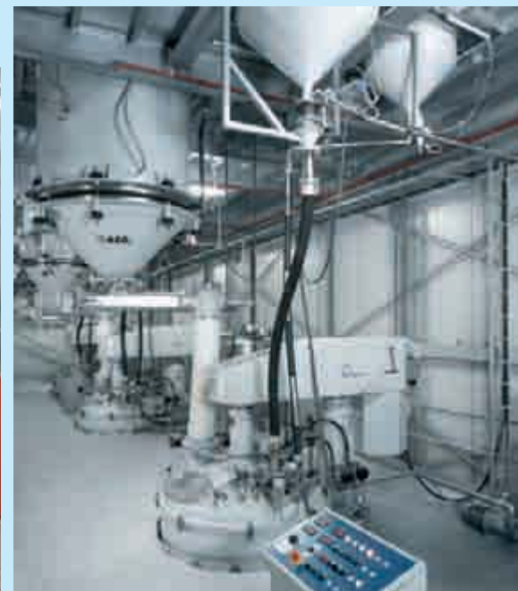
Dissolver feeding in the flour production
