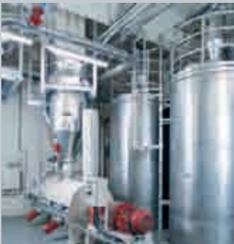
AZO suction weighing systems, the optimum solution for large and medium-sized components
