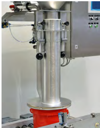
Filling head with elastic sealing surface
