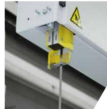
Knife protection unit adjustable by motor
