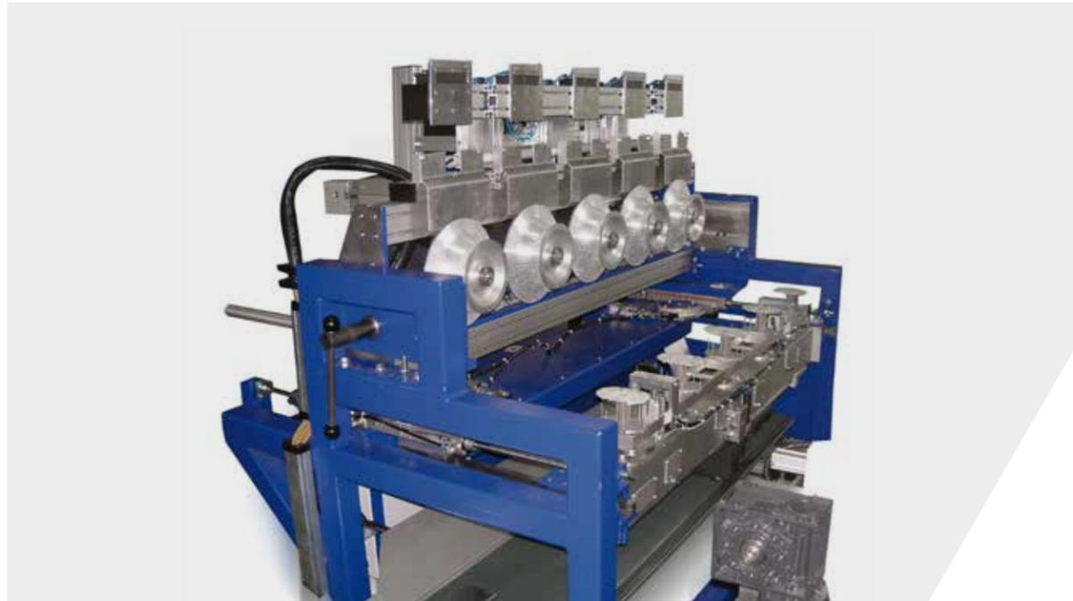
**AUTOMATED SYSTEM FOR MILLING SPONGES IN DIFFERENT GEOMETRIES AND SHAPES. MACHINE PROCESSES FOAM BARS THAT ARE 2 M IN LENGTH.**
