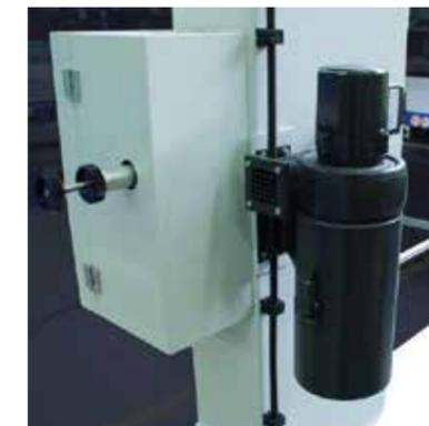
Grinding dust extraction unit
