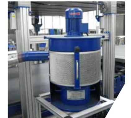
Grinding dust extraction unit
