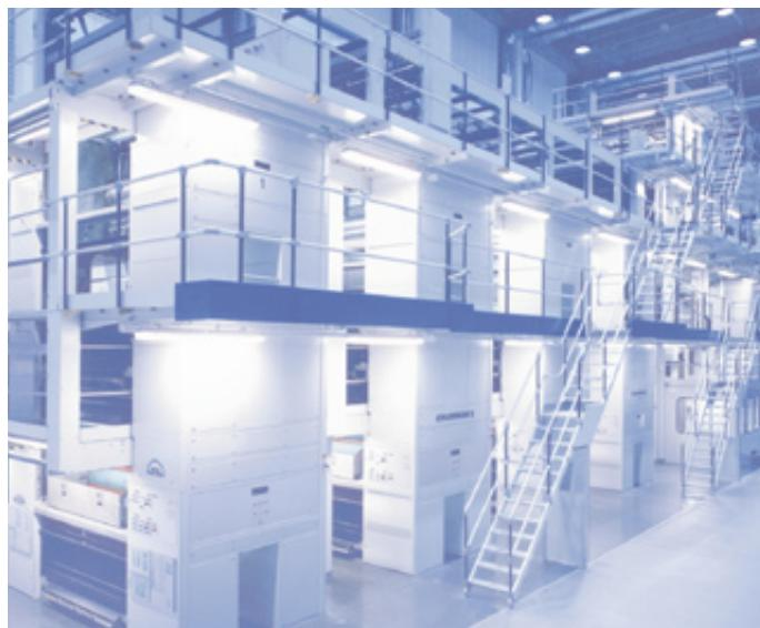
Baumüller was the first system manufacturer in the printing machine sector to perform pioneering work with direct drive technology. In the past, it was more common to drive synchronized rotating cylinders using positive coupling via hard gearing. Increasingly more manufacturers are now relying on direct drive technology with electronic synchronization from Baumüller and are profiting from the advantages.
