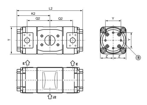
Mounting threads 4 x dimensions 'G' - both ends
