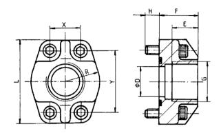
Threaded pipe flanges are spot-faced for pipe fittings.
