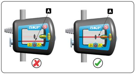
*Fig. 11. Hit the target* A Laser line
