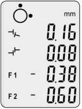
Fig. 19. Measured misalignment
