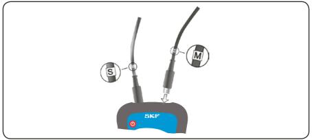
Fig. 9. Connection of the measuring units
