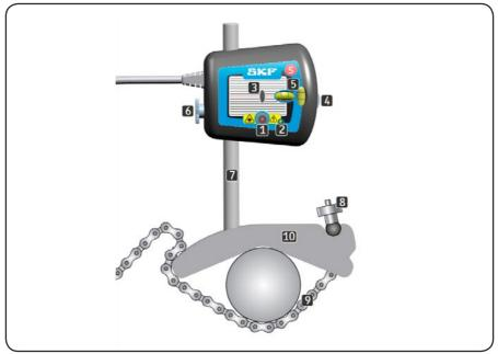
Fig. 7. Mechanical fixture with measuring unit
