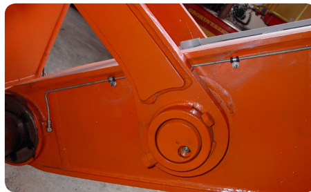
The shielded, galvanized-steel lubricant line at the tip of the hydraulic excavator's stick assures high dependability.
