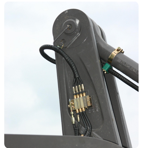
VPKM-4 progressive feeder used supply the TP linkage on Volvo wheel loaders. All the high-pressure hoses are sheathed in wear-proof coils for their protection.
