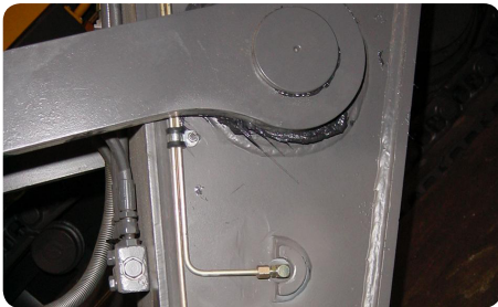
Connection of the stick tip to an EC460B Volvo hydraulic excavator. Welded-on adapters protect the lube point from damage!
