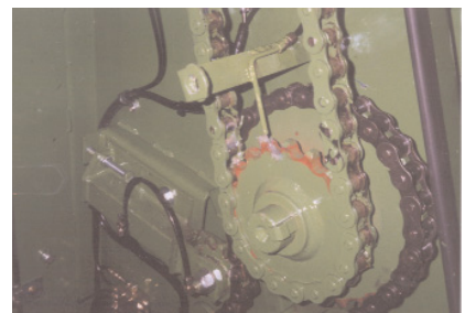
Universal spreader with lubrication of the spreading mechanism's drive chain.
