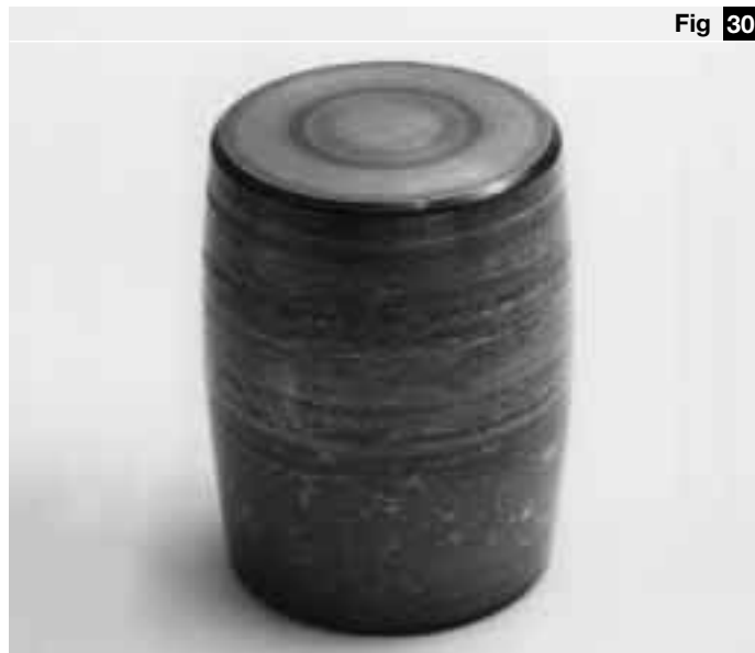
Figs 30 and 31 Smearing normally leads to premature spalling
